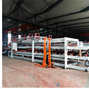
Integrated rollers and forming stations for precise profile shaping.
