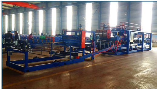
Precision roll forming machinery for Z-lock profile consistency.
