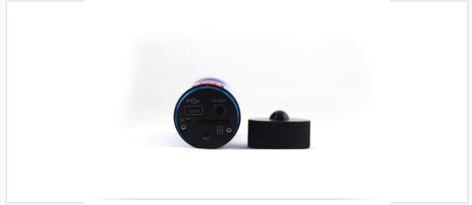
Side panel showing TV output, microphone, and data ports.
