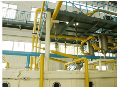
Integrated filtration system for removing impurities from miscella.
