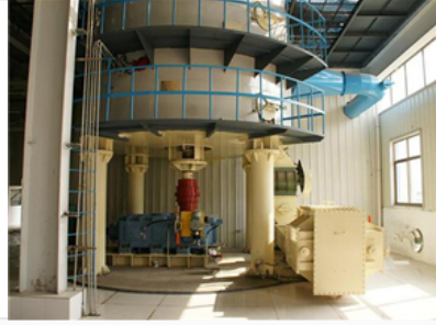
Robust desolventizer unit with heavy-duty support columns.
