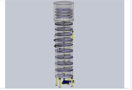
Vertical extraction column optimized for countercurrent extraction.
