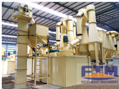
A high-performance ultrafine mill designed for processing minerals into fine powders with integrated dust collection.
