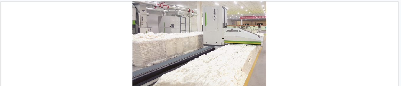
The JWF1011 unit integrated into a textile production line, showing the plucking arm and suction assembly.
