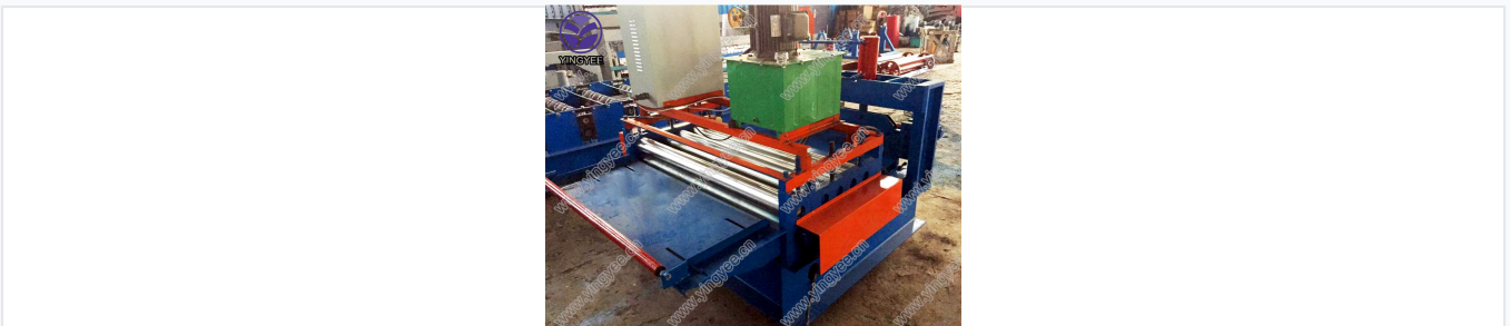
High-precision straightening machine integrating traction and leveling functions.
