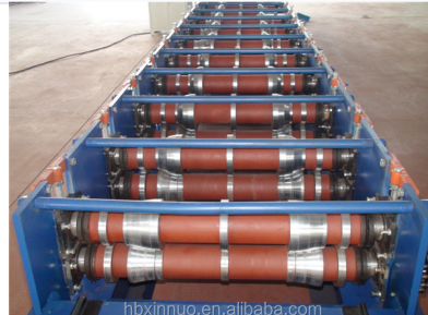
Gradual metal shaping through multiple roller passes
