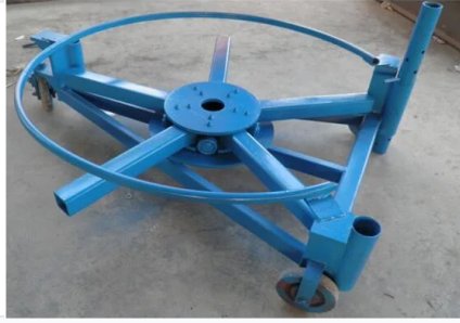
Heavy-duty mobile support frame featuring a central rotating mechanism for even weight distribution during silo construction.
