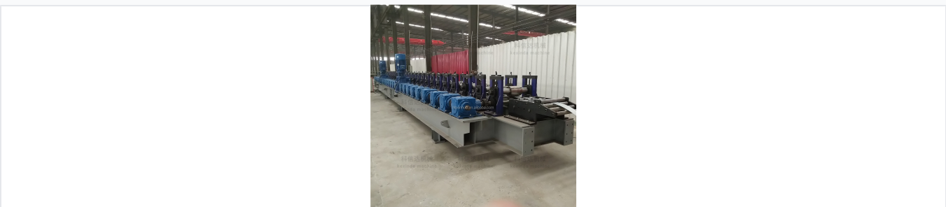
Detailed view of the multi-station roll forming assembly and straightening unit.
