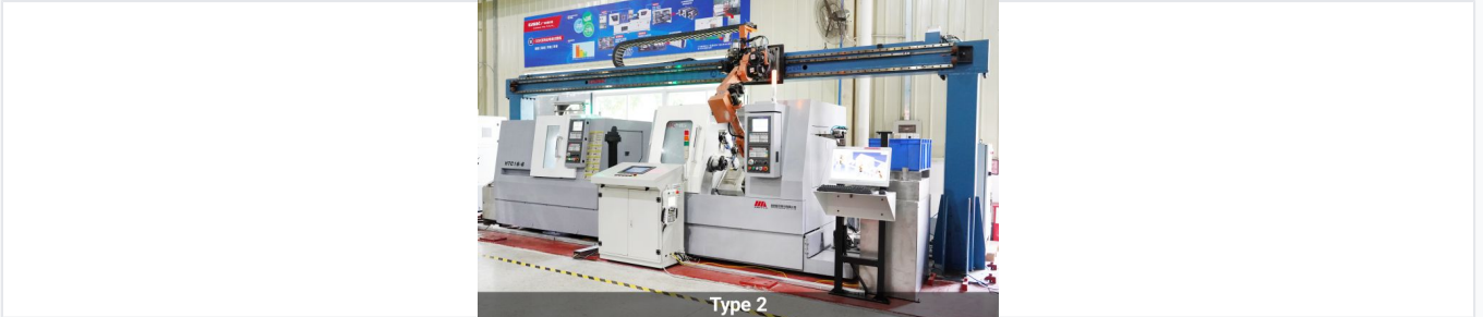
Complete robotic setup integrated with CNC machinery for automated manufacturing.
