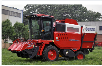
Advanced 4-row harvesting head designed for efficient crop gathering.
