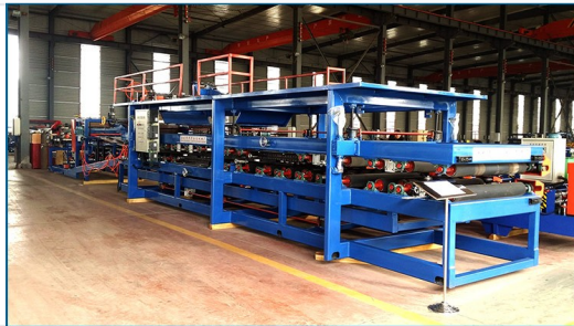
Precision rollers designed for shaping metal sheets into durable profiles.
