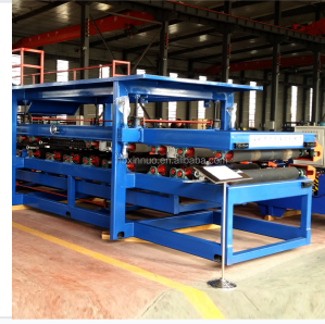
Control station for monitoring and adjusting the roll forming process.
