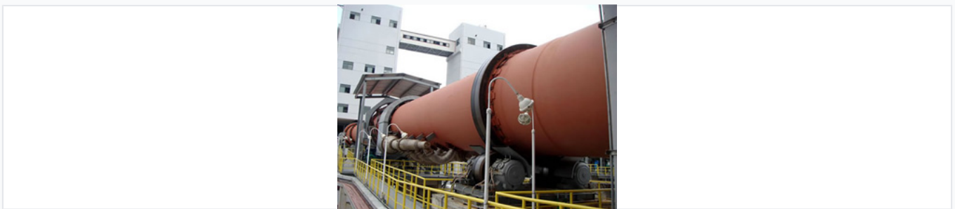
A heavy-duty rotary kiln featuring a rotating cylindrical shell, support rollers, and advanced heat transfer components for efficient calcination.
