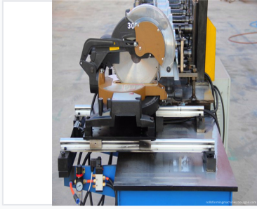
Advanced flying saw cutter system ensures precise length control during high-speed production.
