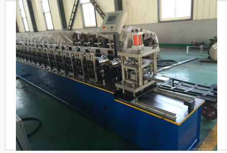
Robust machine frame equipped with multiple stations and adjustable roller molds.
