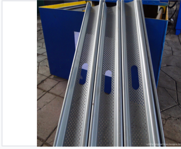
Finished panel sample showing consistent forming quality and optional perforation holes.
