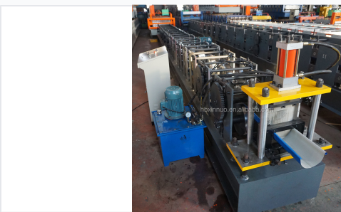
Linear forming path with precision rollers ensures consistent profile shaping and safety.
