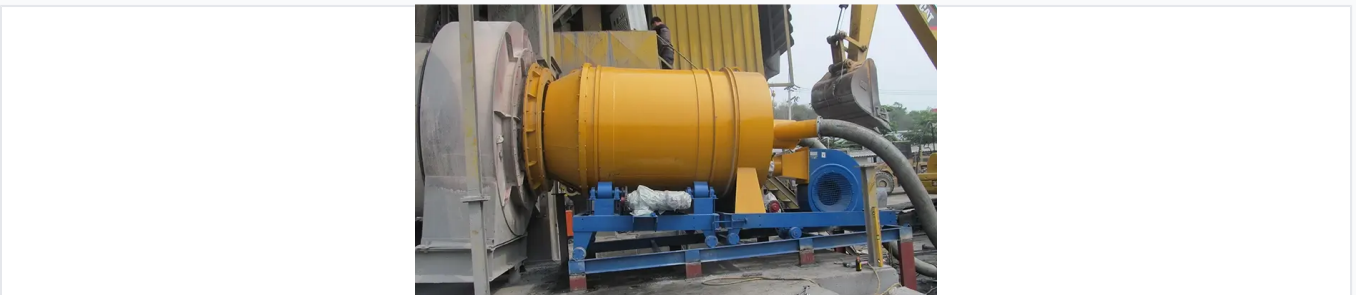
A heavy-duty pulverized coal burner designed for optimal fuel combustion and heat distribution.
