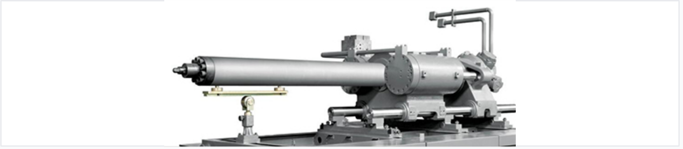
Dual-cylinder injection system designed for accurate and stable operation.
