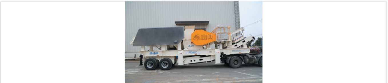
A comprehensive mobile crushing unit designed for primary reduction in various industrial sites.
