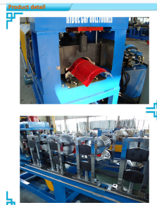
Precision roller arrangement for consistent metal shaping.
