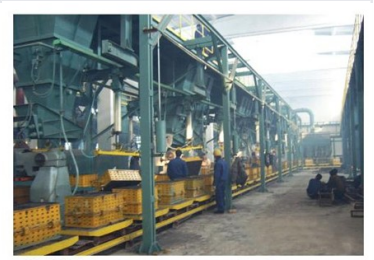
环型造型线 Ring shaped molding line
