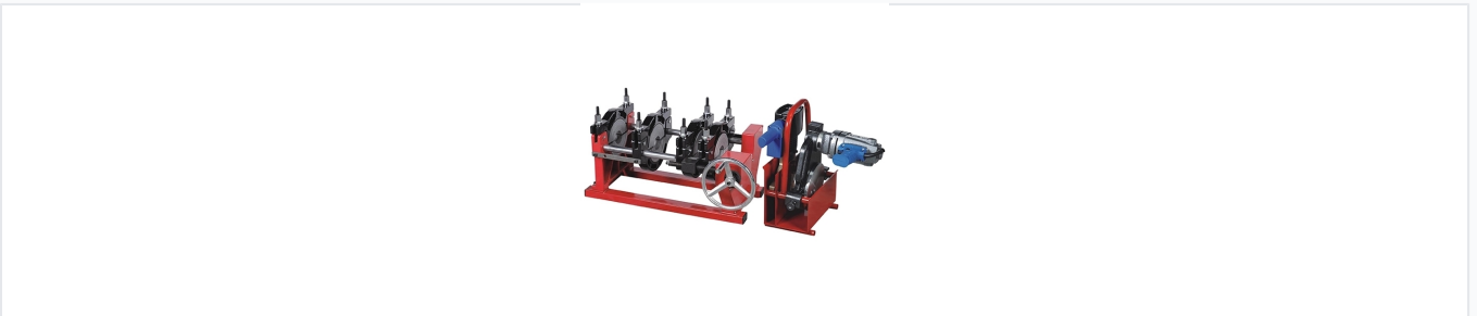
A complete view of the welding system, including the frame, heater, and facer.
