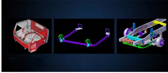
Detailed view of the reinforced chassis and suspension systems.
