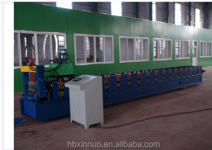
Robust machine construction with multiple forming stations for precise profile shaping.
