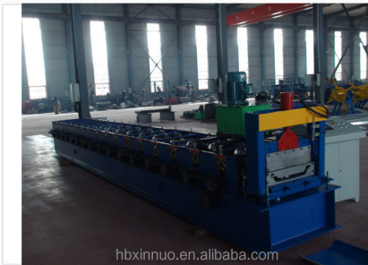
The forming section features a hydraulic cutting system for efficient and clean panel separation.
