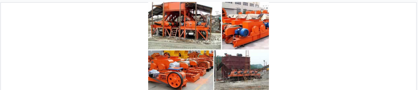
Compression-type crushing mechanism using dual rollers rotating in opposite directions.
