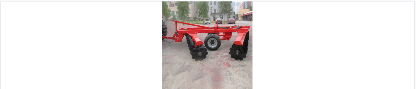
Equipped with a trailing wheel for precise depth control and stability during high-efficiency tilling.
