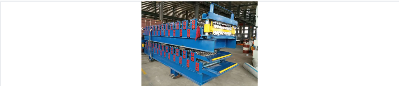
Designed for continuous operation, this machine integrates feeding, forming, and output sections.
