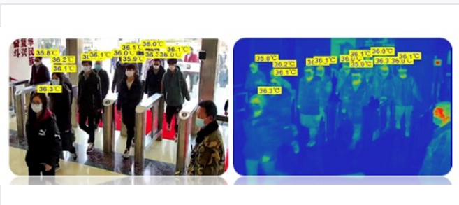
Real-time thermal monitoring interface displaying multiple individuals simultaneously.
