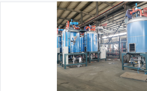
The processing chamber features a stainless steel design for uniform steam distribution.
