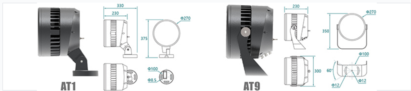
Detailed technical drawing displaying the dimensions for the AT1 model, including diameter and mounting specifications.
