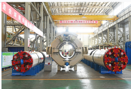
The specialized cutterhead designed for simultaneous boring and pipe installation.
