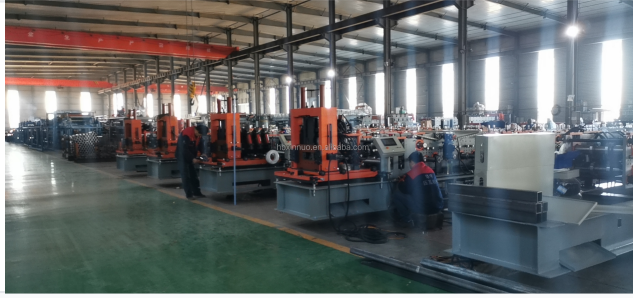
Automated production line featuring multiple forming stations for high-volume purlin manufacturing.
