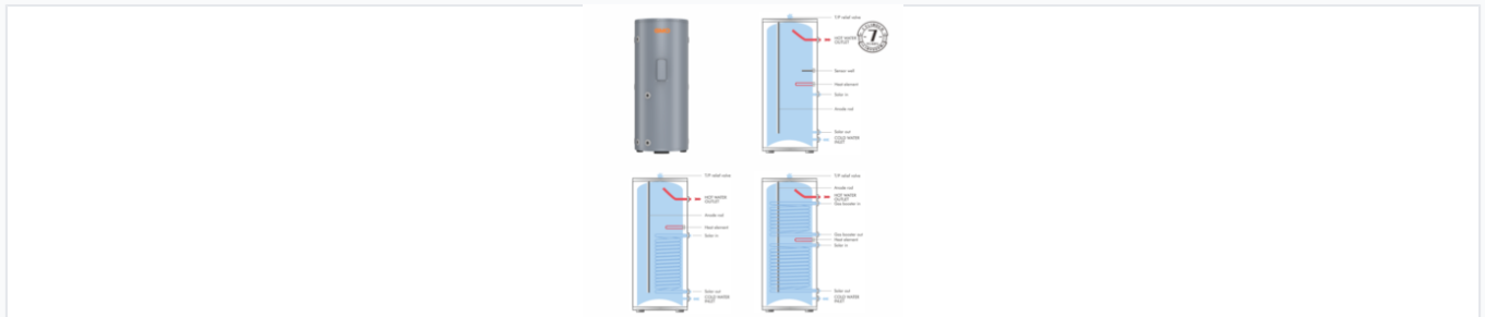
Diagram showing internal components including T/P relief valve, anode rod, and various connection points for solar, gas, and electric systems.
