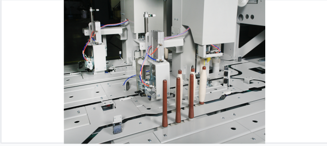
Multi-station configuration designed for high-throughput winding and automated bobbin handling.
