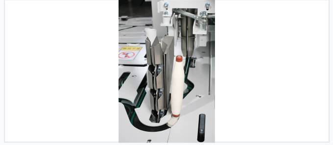
Precision metal guides ensure accurate yarn placement during high-speed winding operations.
