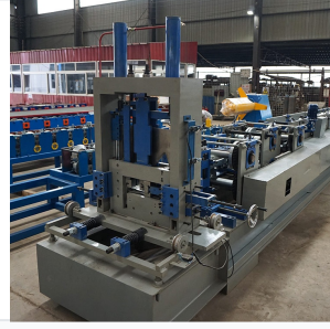
Adjustable components allow for various purlin sizes and thicknesses within the same line.
