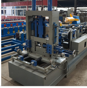
Detailed view of the 18-group roller system designed for C, Z, and U profiles.
