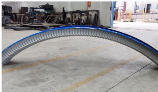
Precision-formed corrugated arch panels with blue trim, ready for assembly into large-span structures.
