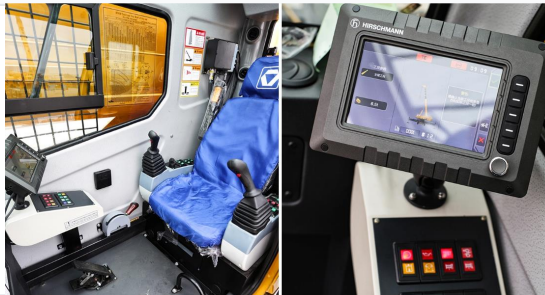
Advanced control console with load monitoring display.
