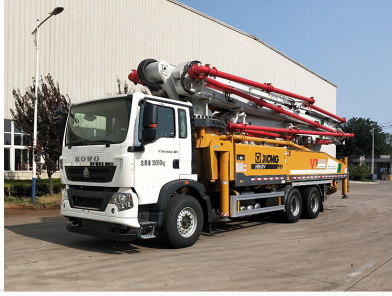
Heavy-duty truck chassis platform for concrete pouring operations.
