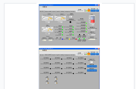
Comprehensive software interface for monitoring cell voltage, SOC, and cycle counts.
