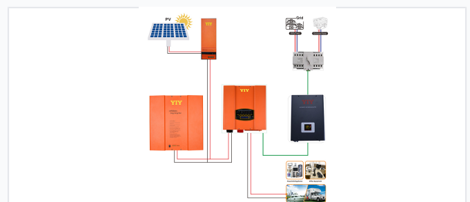
The battery pack connected to PV panels, utility power, and household appliances.
