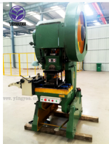
Robust mechanical press featuring a large flywheel for consistent power delivery.
