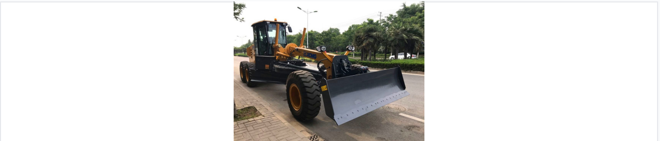
Heavy-duty motor grader performing precise grading operations.
