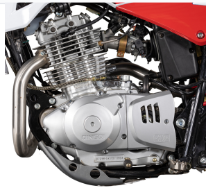
Powerful 250cc oil-cooled EFI engine with balance shaft technology.
