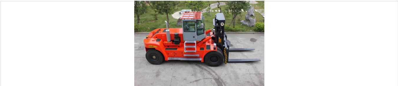
The reinforced mast and hydraulic fork positioner provide precise control for heavy loads.
