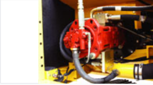
Double pump hydraulic system unit for precise power delivery.
