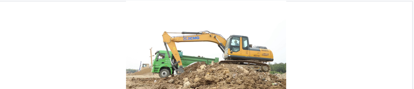
Crawler undercarriage providing stability and maneuverability for earthmoving tasks.
