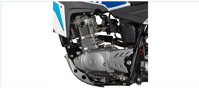
High performance 200cc oil-cooled engine configuration.
