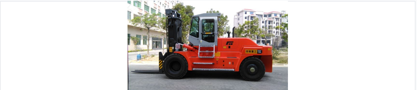
The 18-ton heavy-duty forklift features a reinforced mast and high-capacity hydraulic forks.
