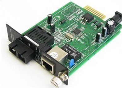
Modular components including fiber media cards and SNMP management modules.
