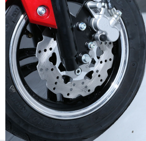
Front wheel assembly featuring a drilled disc brake rotor for heat dissipation.
