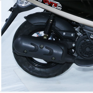
Rear assembly featuring the double-C muffler.
